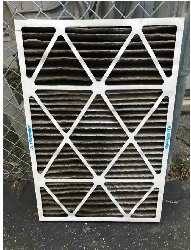
Photo #8: AHU – MERV 8 filter observed moderate loading
