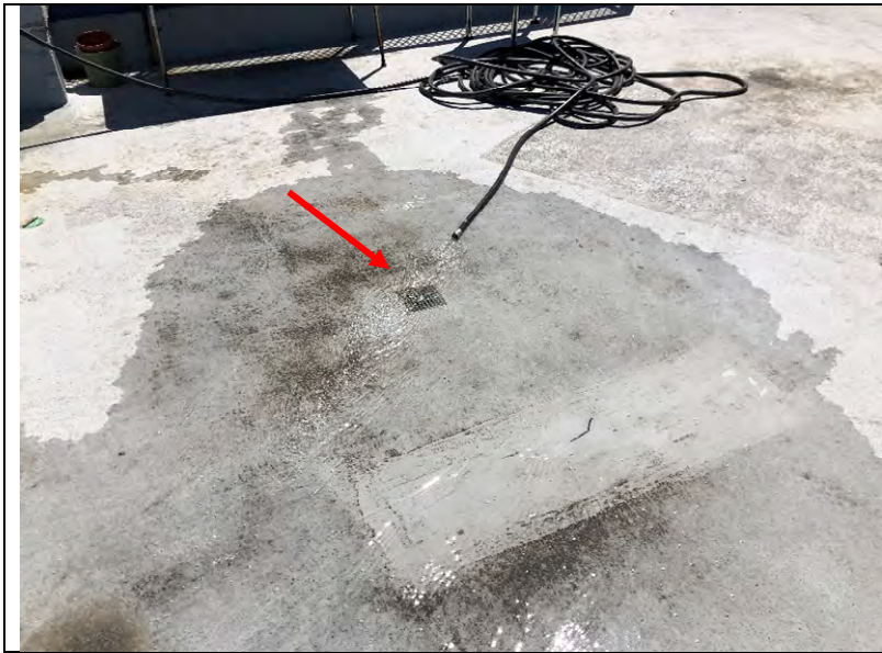
Photo 57: Flood testing outside classroom 555.
