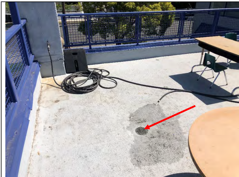
Photo 56: Flood testing at a drain outside of classroom 555.
