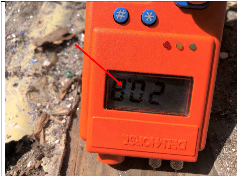
Photo 76: Moisture reading of the wood at the threshold. 20.8 %
