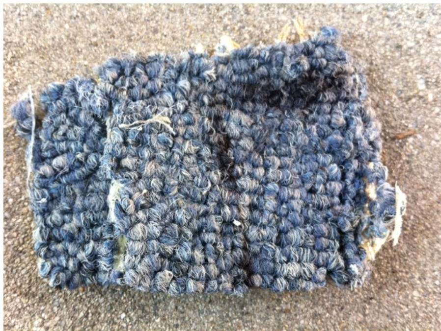
Photo 6 – Carpet sample with suspect mold from Classroom 1; Sample 130920-0255-VMU-B02.
