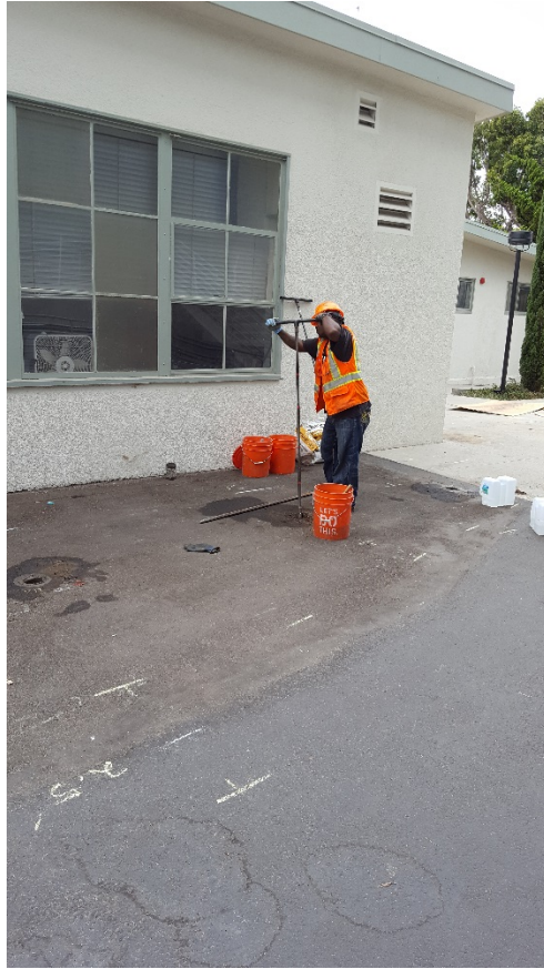
Photo 5 – Hand Auger Sample Collection
