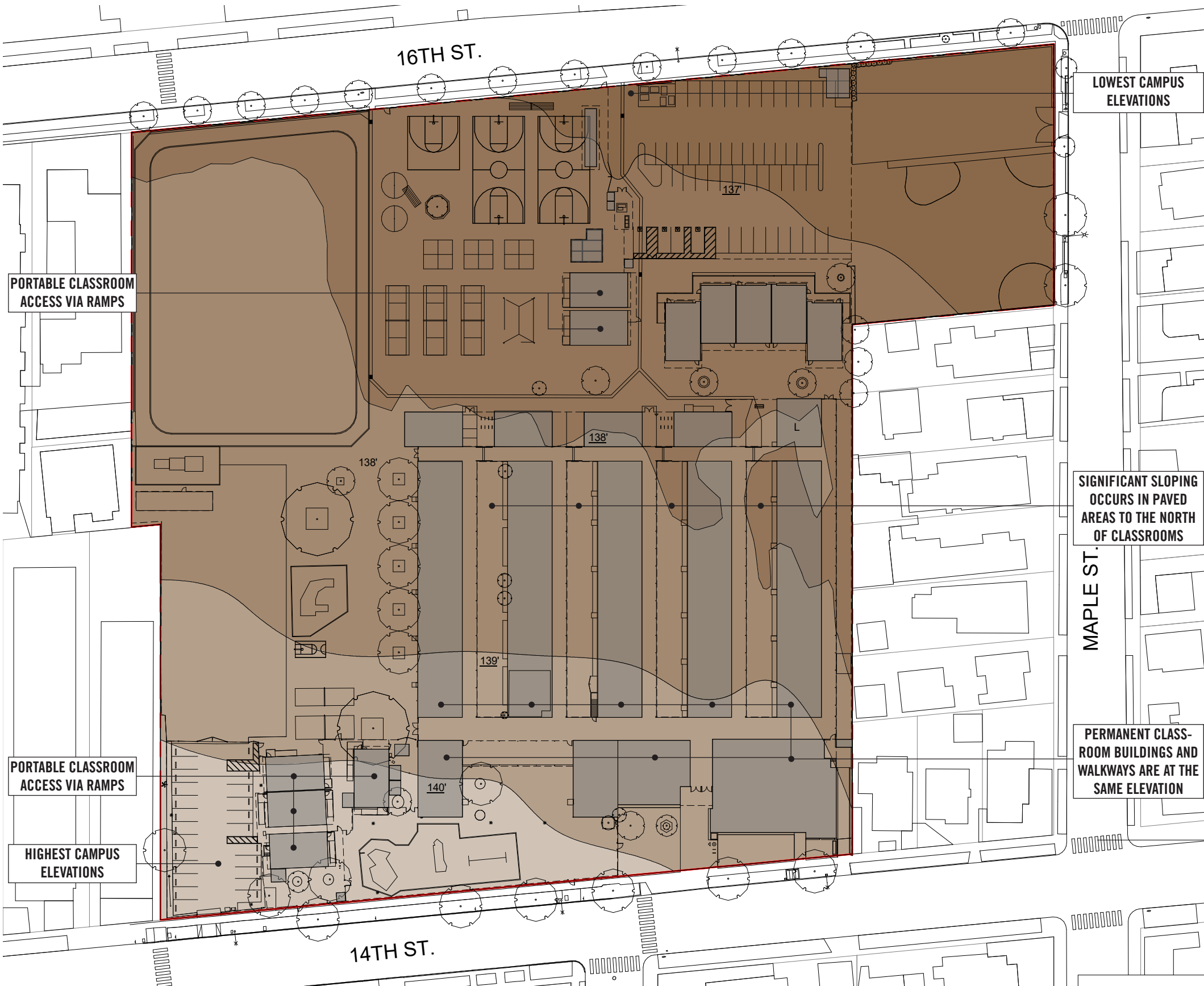
TOPOGRAPHY The minor slope of the site toward the southeast explains the storm water discharge system, but otherwise topography is of little consequence in the planning for this campus.
