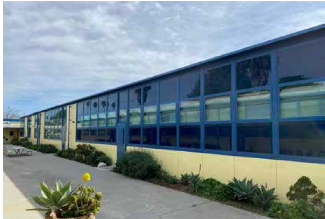
ORIGINAL CLASSROOM BUILDINGS These buildings align with long dimension north south facing, large windows on the north side, circulation and entrances on the south side.
