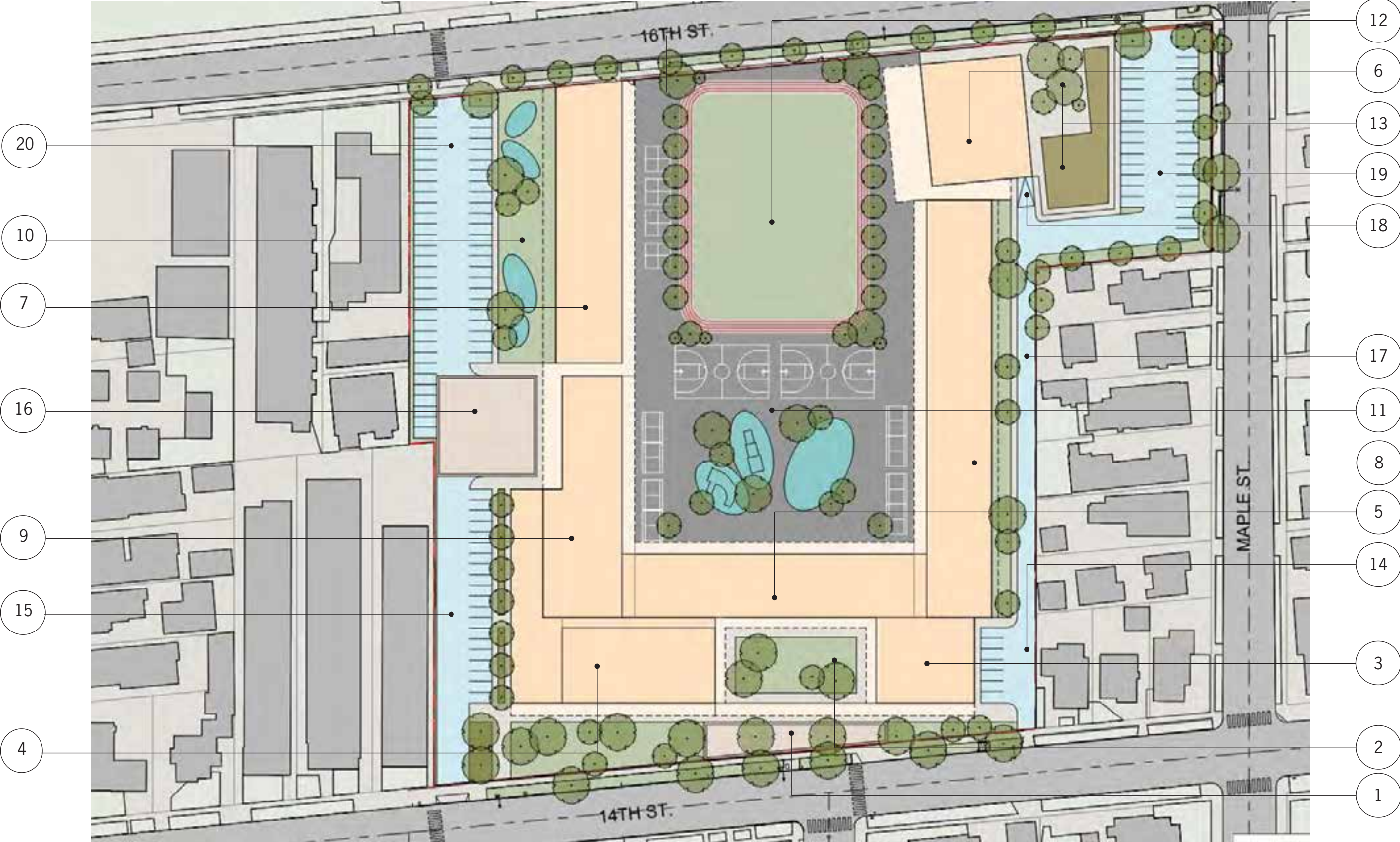
CAMPUS AT COMPLETION The U-shape configuration maintains the front of school on 14th Street, provides for vehicular access across the site on the north and south sides and places outdoor facilities at the heart of campus protected by surrounding school buildings.
