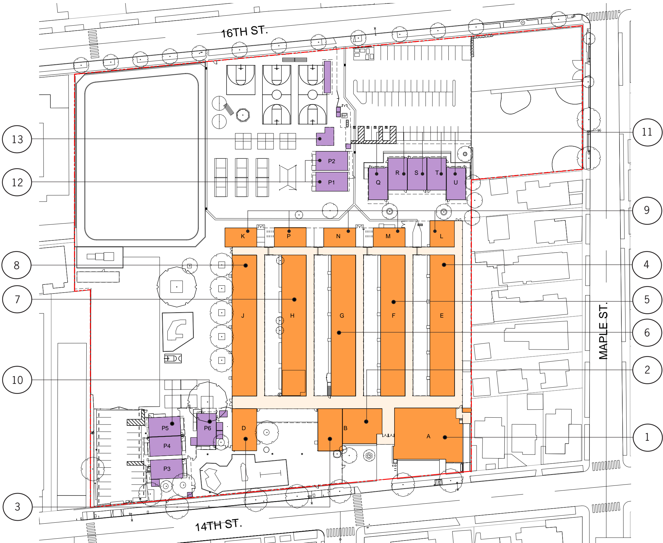
BUILDING FOOTPRINTS All buildings on campus are one story in height, most permanent buildings arranged as linear classrooms buildings in the east west orientation for ideal north south solar orientation. Additional classrooms occupy the east end of the complex, common facilities the west end facing onto 14th Street.
