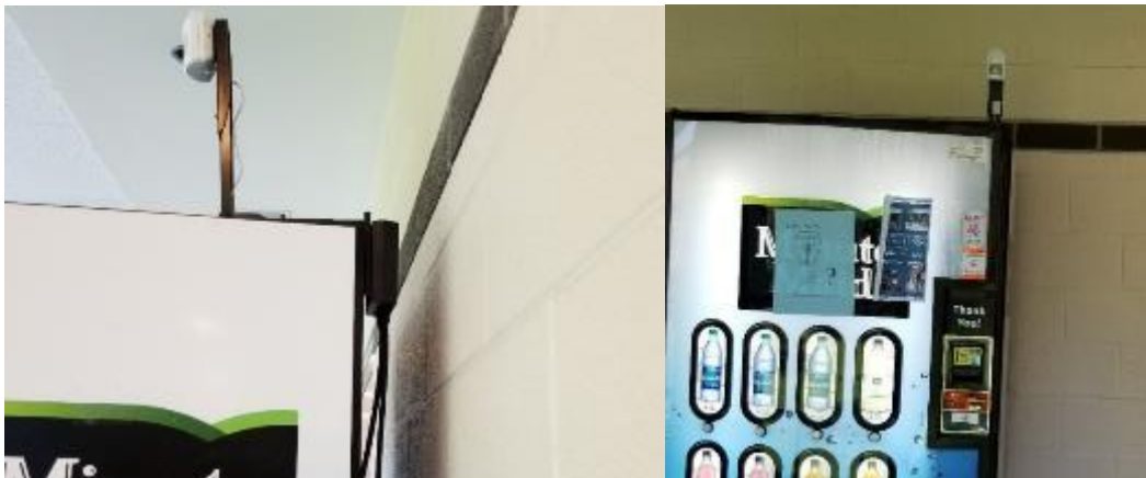
Figure 1. Vending misers retrofitted on vending machines at another District. Vending misers reduce energy consumption by turning off the machine when no motion is sensed for 15 minutes (turning on at regular 90-minute intervals to ensure the product remains cold).
