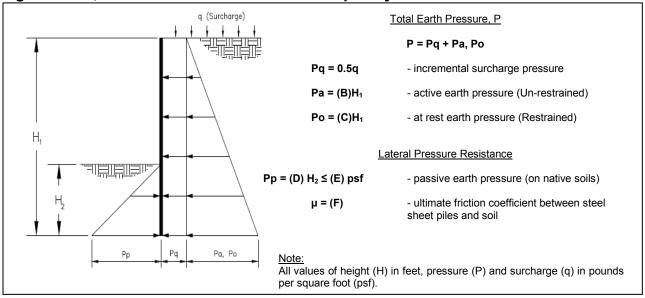
Figure No. 9, Lateral Earth Pressures on Temporary Cantilever Wall
