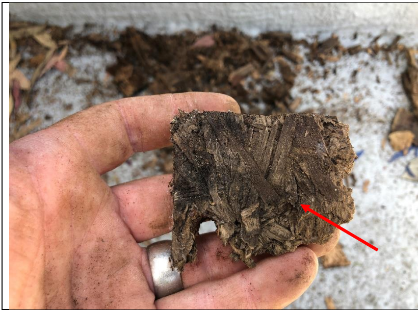
Photo 347: Deteriorated OSB material that fell from under the coping cap at the handrail curbs during observations.
