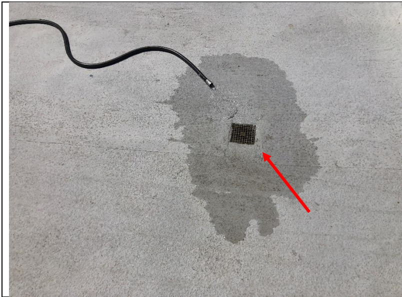
Photo 58: Flood testing a drain on the elevated walkway.
